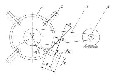
Fig. 1. Scheme of the hammer crusher rotor
